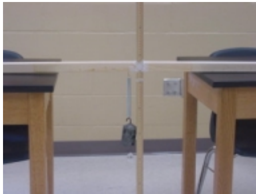
Figure 3: Illustration of setup for Hooke's Law activity
