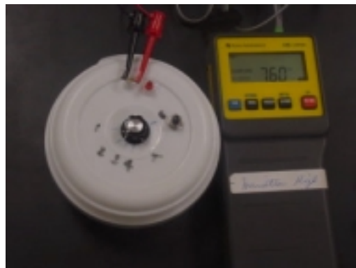
Figure 2: Ohm's law apparatus with voltmeter
